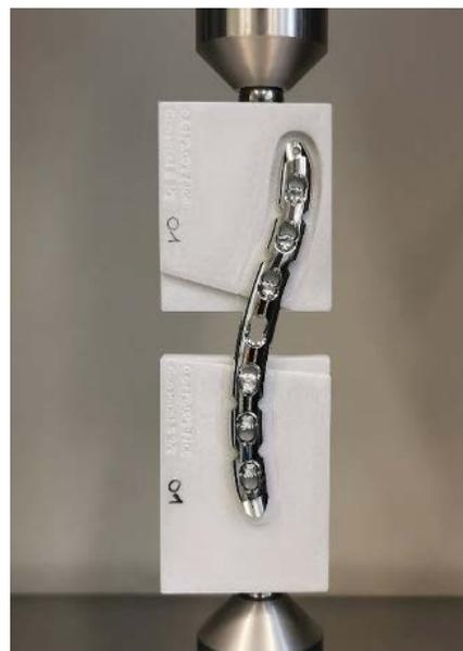
**Figure 3** Exemplary test setup for the 3.5 LCP Superior Plate (SS).
