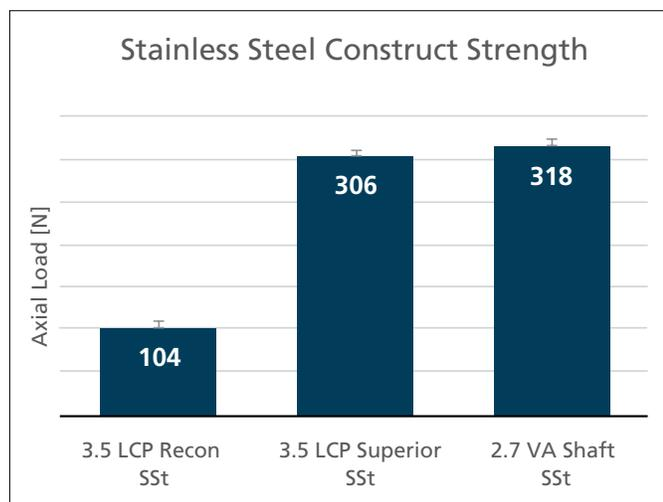
Figure 4a Construct strength results for static load-to-failure tests.
