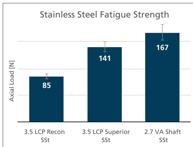
Figure 5a Construct fatigue strength results for cyclic tests (at 1,000,000 cycles).
