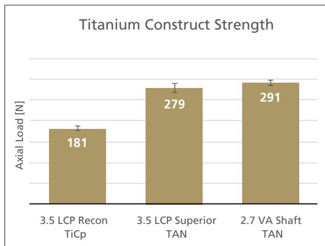
Figure 4b Construct strength results for static load-to-failure tests.
