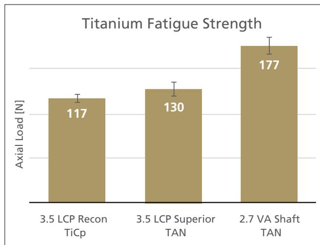
Figure 5b Construct fatigue strength results for cyclic tests (at 1,000,000 cycles).
