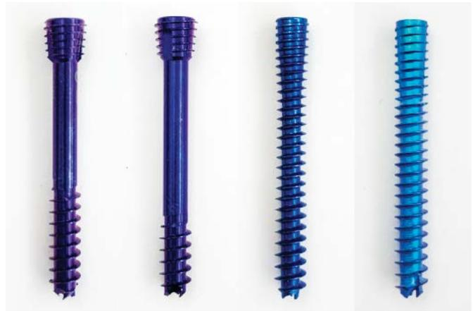
**Figure 1** Representative screws tested (left to right): DePuy Synthes CCHS Short Thread, DePuy Synthes CCHS Long Thread, Acumed Acutrak 2, Arthrex Compression FT.
