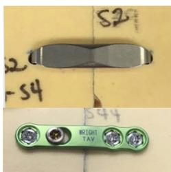
The constructs were prepared from custom 25 mm x 25 mm bicortical Sawbones® blocks. The constructs consisted of two blocks of similar dimensions with each matching surface milled flat and sanded with 600 grit abrasive paper in order to obtain flat, smooth surfaces. The
