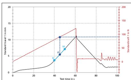
**Figure 2:** Example output data for Groups 1 and 2. Slope calculated between points B and M to find the inflection point (IP) at which the displacement equals the pitch rate. The corresponding load at that point is the load required for the screw to self-tap.
