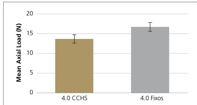
Figure 5: Group 2 – Ø4.0 mm CCHS vs Ø4.0 mm Stryker Fixos into 20 pcf foam
