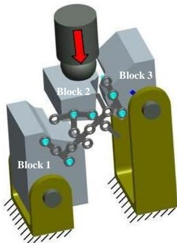
**FIGURE 3.** Mechanical three-point bend test model.
