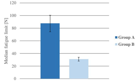
**FIGURE 7.** Median fatigue limit and standard deviation shown for both groups. The difference between group A and B was found to be statistically significant ( $p < 0.05$ ).
