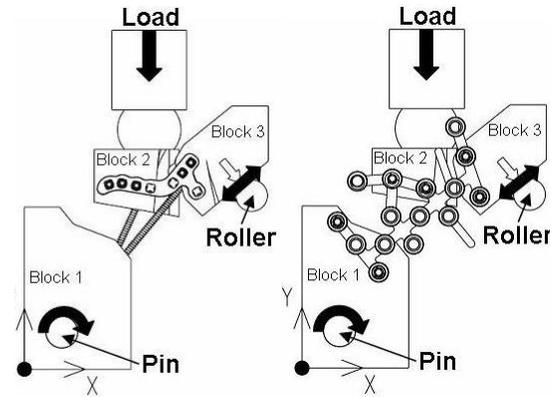
**FIGURE 6.** Mechanical test setup for group A (left) and group B (right).
