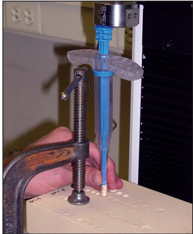
**Figure.** The harvested plugs were placed in the delivery tube, aligned above the recipient site in the foam block, and driven into the recipient hole by the Instron actuator using a single impaction.
