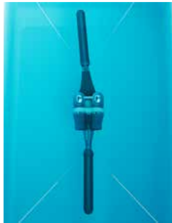
Figure 8: Worst-case construct submersed in a copper sulphate solution according to ASTM F2119. 20
