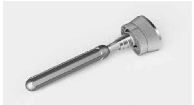
Figure 7: Worst-case femoral (left) and tibial (right) constructs used for displacement force/torque testing. 20
