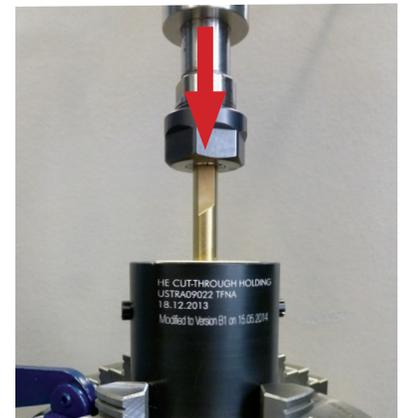
Fig. 4: Test setup with nail construct sample mounted for mechanical testing. Arrow denotes loading direction.
