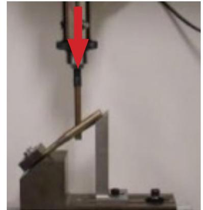
Fig. 3: Test setup with nail construct sample (ex. TFNA Nail) mounted for mechanical testing. Arrow denotes loading direction.
