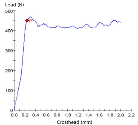
Fig. 4: Representative load displacement curve showing determination of slippage load (P). Shown is a pre-conditioning data set for the TFNA Nail.
