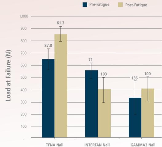
Fig. 6: Results comparison of pre-conditioning and post-conditioning static slippage loads for each nailing system.<sup>1</sup>
