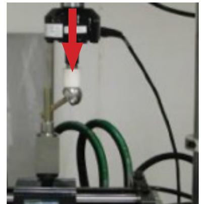
Fig. 5: Implant conditioning test setup with nail construct sample (ex. TFNA Nail) mounted for mechanical testing. Arrow denotes loading direction.
