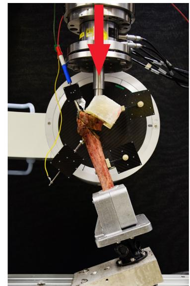
Fig. 6 Test setup with nail construct sample mounted for biomechanical cadaveric testing. Arrow denotes loading direction.
